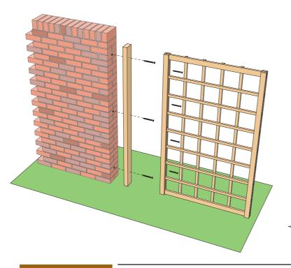
Fix a vertical batten to the wall using screws and wall plugs, the batten should be the same length as the trellis.
