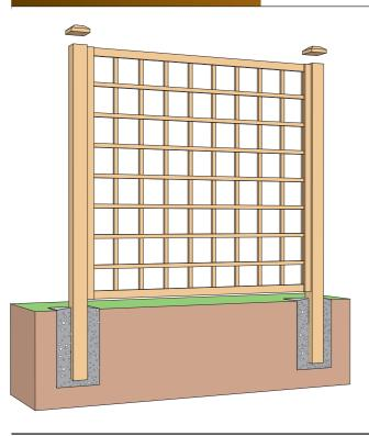
To use trellis as a free standing feature or decorative fence it will be necessary to support it using posts fixed into the ground.
