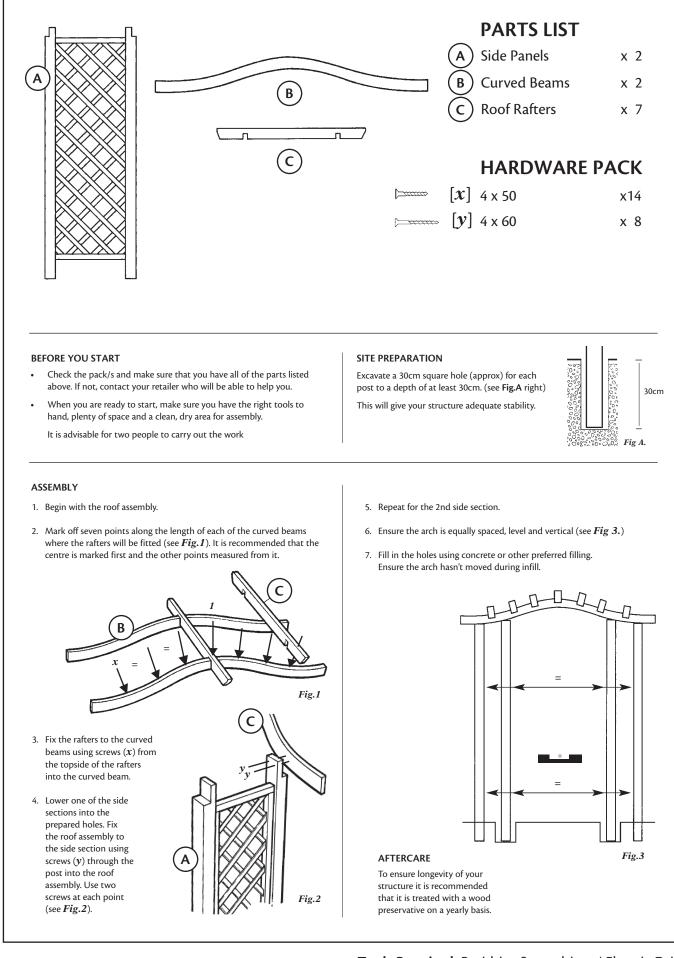
Tools Required: Posidrive Screwdriver / Electric Drill
