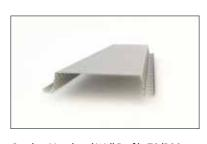
Cembrit Ventilated Wall Profile 70/100 25x70/100mm Horizontal ventilation 1mm steel profile. Used as an alternative to timber battens
